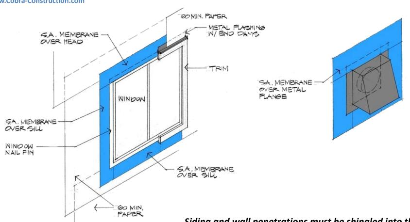
Siding and wall penetrations must be shingled into the building envelope system. This includes windows, dryer vents and all other penetrations. This illustration depicts the concept. Actual conditions may vary.
